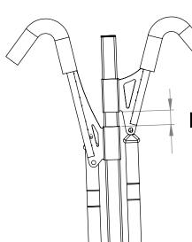
NOTE. There MUST be a gap between the hooks. Adjust position of pivoting post if necessary.
